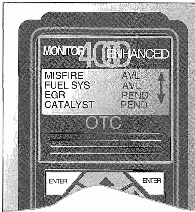
Fig. 6-5. Until all the monitors have had a chance to test the system, you won't know if the OBD II monitoring system will approve the repair.
