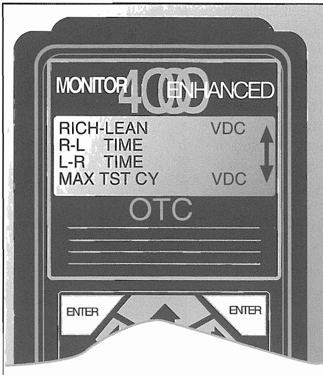
Fig. 3-6. Whether it's a graphic display of sensor activity, or numeric values displayed on a scan tool, the oxygen sensor monitor tests display can save you a lot of troubleshooting time.
