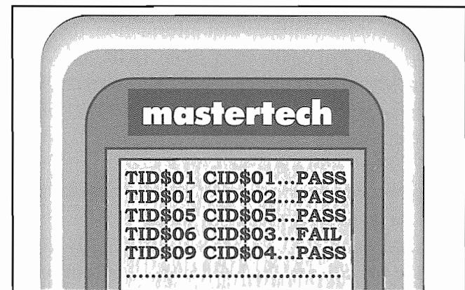
Fig. 3-8. The Non-Continuous monitor display provides information about the current status of individual monitors and individual components providing information to those monitors.
