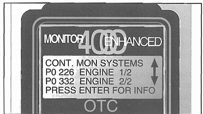
Fig. 3-10. This scanner display of Continuous Monitor tests tells us which controller is reporting the DTCs and how many DTCs are stored.
