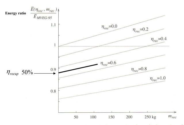
Energy demand in the MVEG-95 cycle of a vehicle equipped with a recuperation device with mass  $m_{rec}$  and efficiency  $\eta_{rec}$ , normalized by the energy  $\bar{E}_{MVEG-95}$  consumed by a vehicle without recuperation device. The example is valid for a vehicle with the parameters  $\{A_f \cdot c_d, c_r, m_v\} = \{0.7 \text{ m}^2, 0.012, 1500 \text{ kg}\}.$
