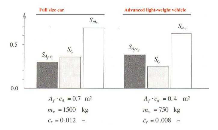
Sensitivities (2.32) of the mechanical energy consumption in the MVEG– 95 cycle with respect to the three main vehicle parameters. Two cases: full-size car (left); advanced light-weight vehicle (right).
