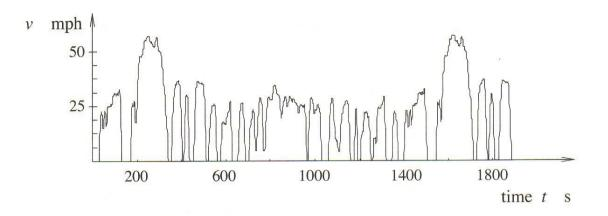
US test cycle FTP-75 (Federal Test Procedure), length: 11.12 miles (17.8 km), duration: 1890 s, average speed: 21 mph (9.43 m/s).
