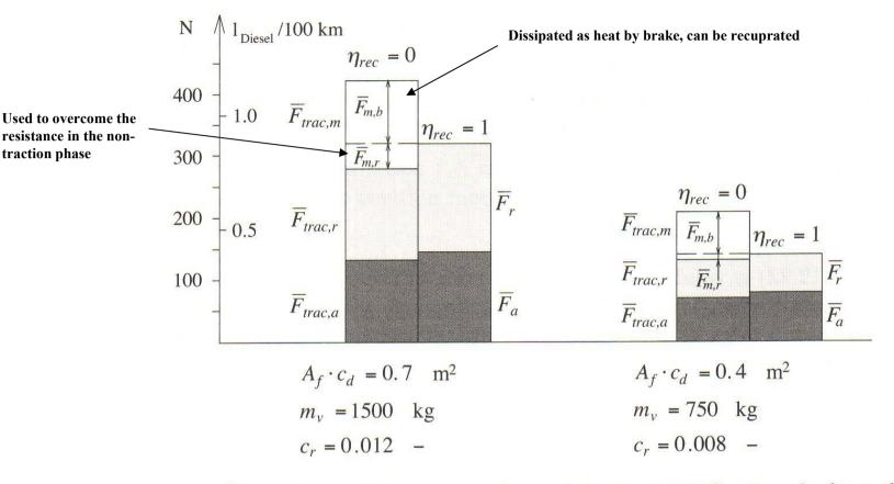
Comparison of the energy demand in the MVEG-95 cycle for a full-size car (left) and a light-weight car (right). A mean force of 1 N is equivalent to 27.78 Wh mechanical energy per 100 km. The lower heating value for Diesel fuel is approximately 10 kWh/l.
