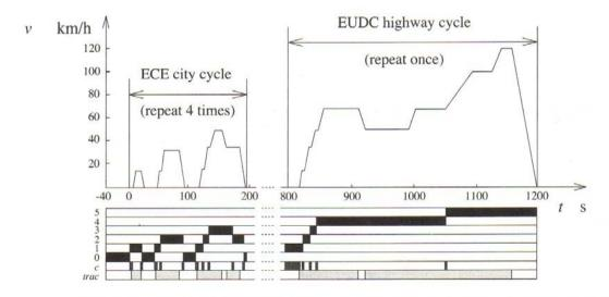
European test cycle MVEG–95, gears 1–5, "c": clutch disengaged, "trac": traction time intervals. Total length: 11.4 km, duration: 1200 s, average speed: urban 5.12 m/s, extra-urban 18.14 m/s, overall 9.5 m/s. The cycle includes a total of 13 gear shifts.
