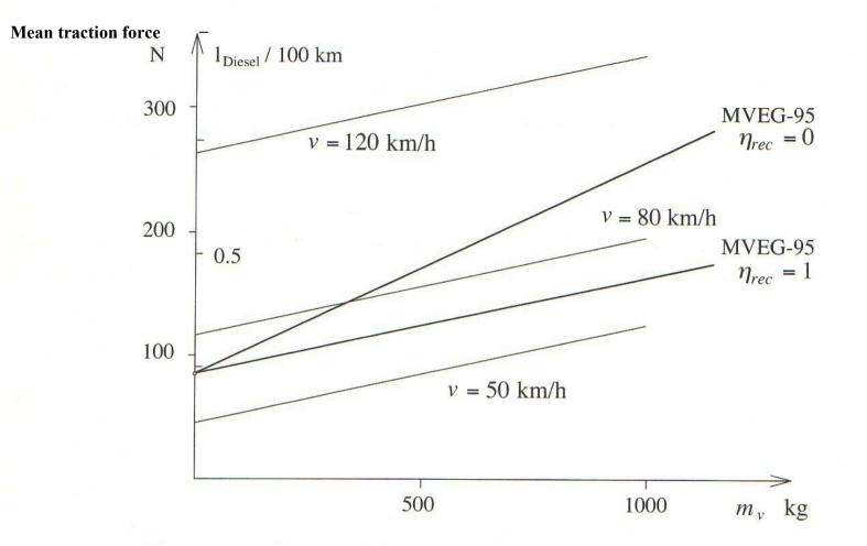
the mean force on the vehicle mass for the MVEG– 95 and three values of speed. The example is valid for an advanced vehicle with the parameters  $\{A_f \cdot c_d, c_r\} = \{0.4 \text{ m}^2, 0.008\}.$
