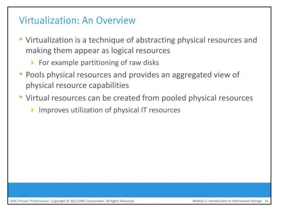
Virtualization is a technique of abstracting physical resources, such as compute, storage, and network, and making them appear as logical resources. Virtualization existed in the IT industry for several years and in different forms. Common examples of virtualization are virtual memory used on compute systems and partitioning of raw disks.
