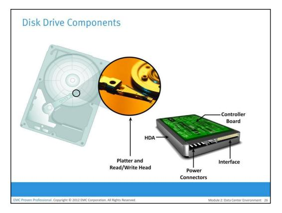
The key components of a hard disk drive are platter, spindle, read-write head, actuator arm assembly, and controller board. I/O operations in a HDD is performed by rapidly moving the arm across the rotating flat platters coated with magnetic particles. Data is transferred between the disk controller and magnetic platters through the read-write (R/W) head which is attached to the arm. Data can be recorded and erased on magnetic platters any number of times.
