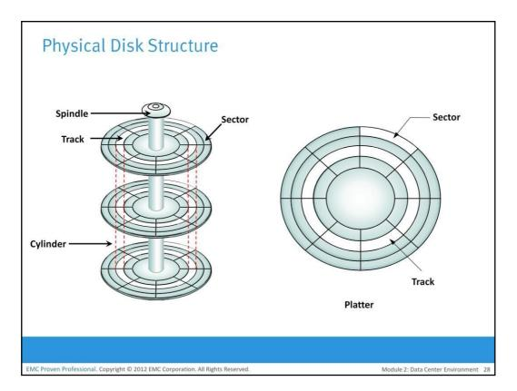
Data on the disk is recorded on *tracks*, which are concentric rings on the platter around the spindle. The tracks are numbered, starting from zero, from the outer edge of the platter. The number of *tracks per inch* (TPI) on the platter (or the *track density*) measures how tightly the tracks are packed on a platter.
