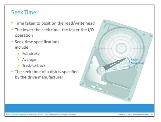
The *seek time* (also called *access time*) describes the time taken to position the R/W heads across the platter with a radial movement (moving along the radius of the platter). In other words, it is the time taken to position and settle the arm and the head over the correct track. Therefore, the lower the seek time, the faster the I/O operation. Disk vendors publish the following seek time specifications:
