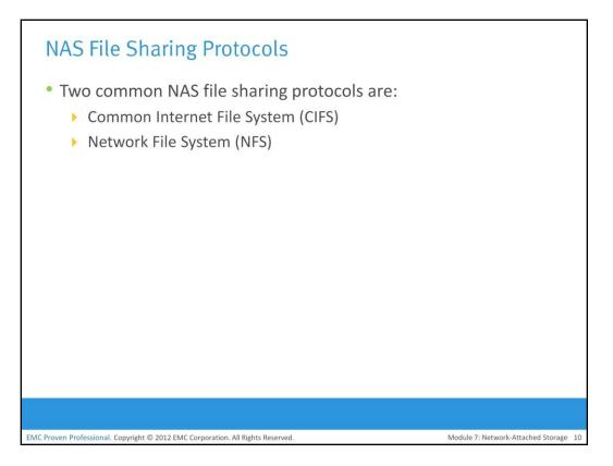
Most NAS devices support multiple file-service protocols to handle file I/O requests to a remote file system. As discussed earlier, NFS and CIFS are the common protocols for file sharing. NAS devices enable users to share file data across different operating environments and provide a means for users to migrate transparently from one operating system to another.
