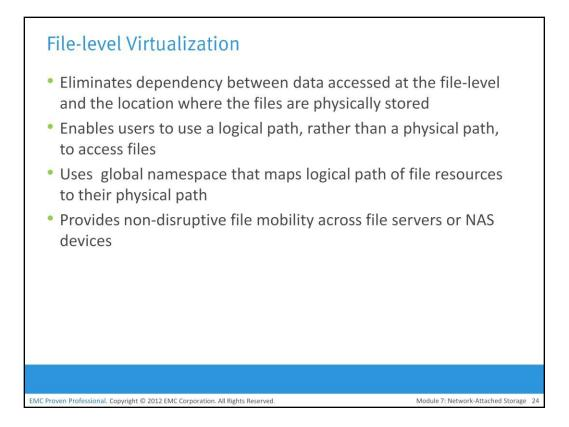
A network-based file sharing environment is composed of multiple file servers or NAS devices. It might be required to move the files from one device to another due to reasons such as cost or performance. File-level virtualization, implemented in NAS or the file server environment, provides a simple, nondisruptive file-mobility solution.
