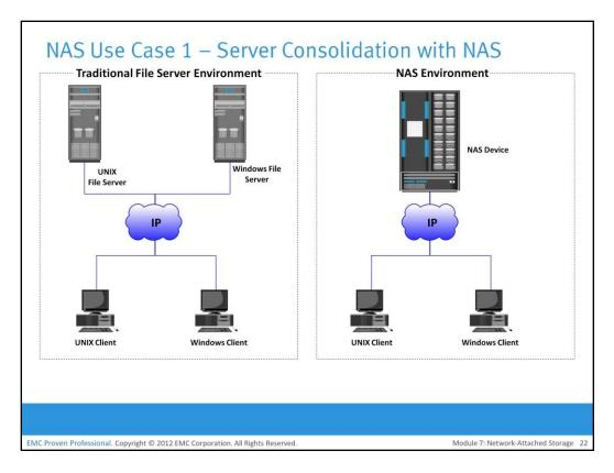
The slide provides a use case that illustrates how a NAS enables consolidation of file servers.
