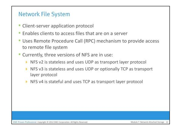
Network File System (NFS) is a client-server protocol for file sharing that is commonly used on UNIX systems. NFS was originally based on the connectionless User Datagram Protocol (UDP). It uses a machine-independent model to represent user data. It also uses Remote Procedure Call (RPC) as a method of inter-process communication between two computers. The NFS protocol provides a set of RPCs to access a remote file system for the following operations:
