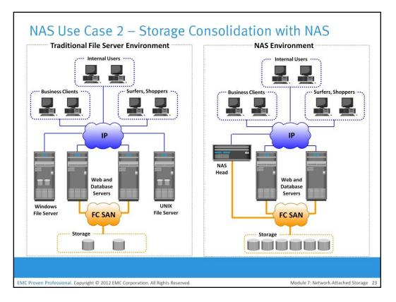
The slide provides another use case that shows how storage resources in a traditional file server environment can be consolidated using NAS.
