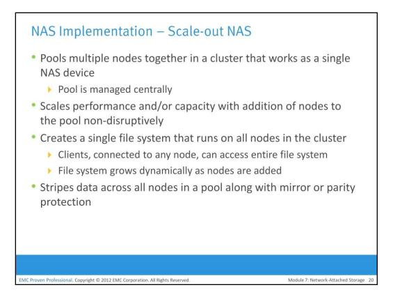
The scale-out NAS implementation pools multiple nodes together in a cluster. A node may consist of either the NAS head or storage or both. The cluster performs the NAS operation as a single entity.
