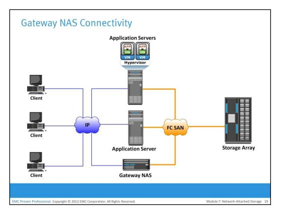
In a gateway solution, the front-end connectivity is similar to that in a unified storage solution. Communication between the NAS gateway and the storage system in a gateway solution is achieved through a traditional FC SAN. To deploy a gateway NAS solution, factors, such as multiple paths for data, redundant fabrics, and load distribution, must be considered.
