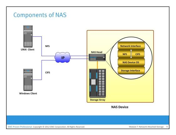
A NAS device has two key components: NAS head and storage. In some NAS implementations, the storage could be external to the NAS device and shared with other hosts. The NAS head includes the following components:
