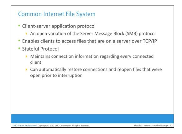
Common Internet File System (CIFS) is a client-server application protocol that enables client programs to make requests for files and services on remote computers over TCP/IP. It is a public, or open, variation of Server Message Block (SMB) protocol.
