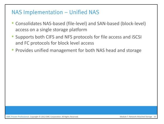
The unified NAS consolidates NAS-based and SAN-based data access within a unified storage platform and provides a unified management interface for managing both the environments.
