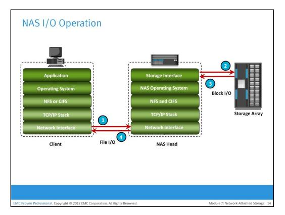
NAS provides file-level data access to its clients. File I/O is a high-level request that specifies the file to be accessed. For example, a client may request a file by specifying its name, location, or other attributes. The NAS operating system keeps track of the location of files on the disk volume and converts client file I/O into block-level I/O to retrieve data. The process of handling I/Os in a NAS environment is as follows:
