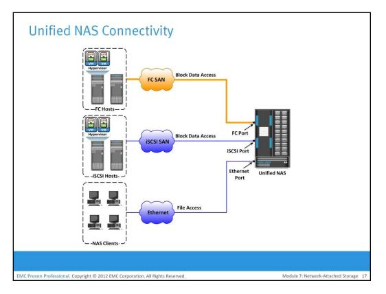
Each NAS head in a unified NAS has front-end Ethernet ports, which connect to the IP network. The front-end ports provide connectivity to the clients and service the file I/O requests. Each NAS head has back-end ports, to provide connectivity to the storage controllers.
